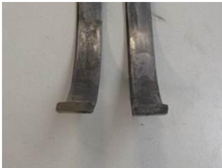
Wear of the locking ring around the load bearing corners
