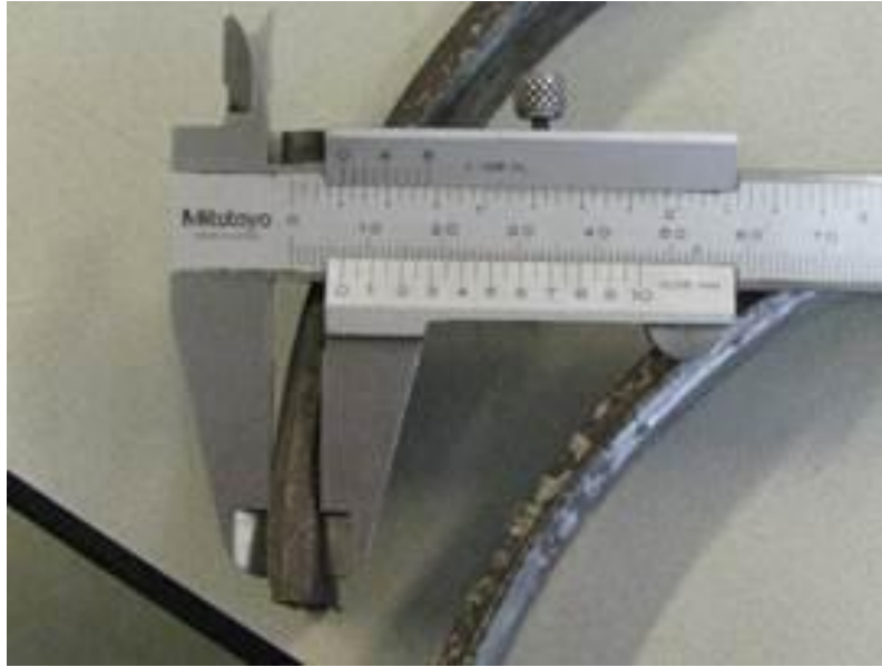
Reduced thickness of the rings.
