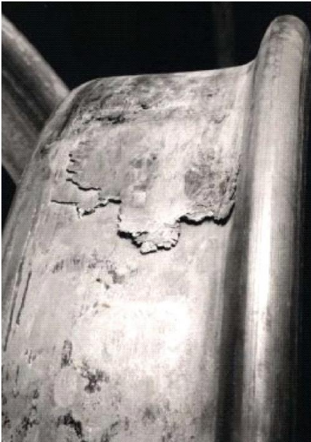
Metal build up on the tread
